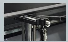
The support units prevent long material from sagging from their own weight to ensure high speed cutting with high accuracy.
