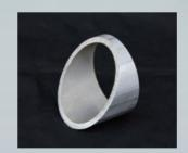
The laser head B-axis provides the ability to perform high accuracy bevel cutting.
